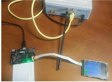
**Fig. 40.** Setup for TEMPEST attack on WooKey
