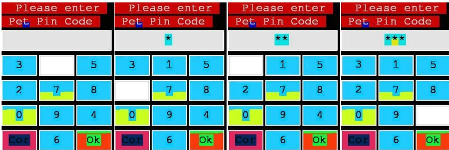
Fig. 35. Capturing '1234' sequence entered on the pinpad
