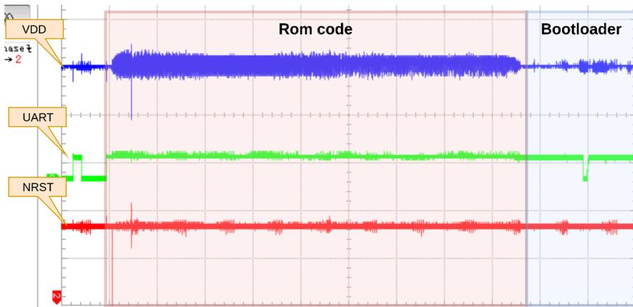
Fig. 9. Boot components timings
