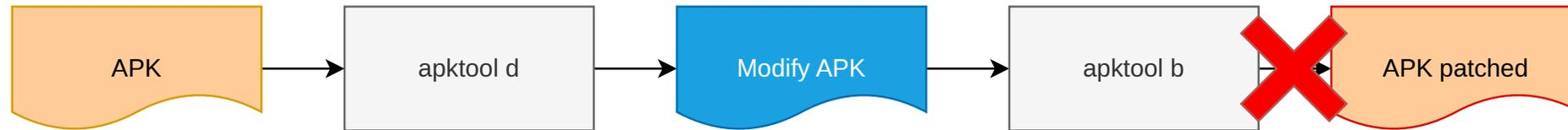
Apktool can't rebuild the application without these lost link.
